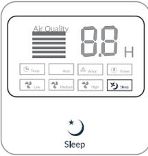
Press the Sleep button on the unit or remote to put the purifier in sleep mode. In sleep mode, the unit will run at a whisper-quiet speed with the lights off, and the smart sensor will turn off. If you would like to have the lights off while operating in other fan modes, then just press the Light button in your preferred mode and the lights will shut off. Press any of the buttons to exit sleep mode.
