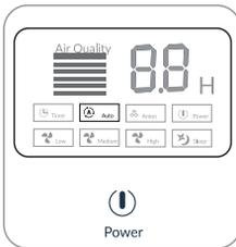
Plug in the purifier. The red power indicator will light up. Use the Power button on the unit or remote to turn on/off. The purifier will start in AUTO mode and the smart sensor will automatically initiate when the unit is turned on. The unit will adjust the fan speed automatically, beginning in high for a few minutes and moving down as needed.
