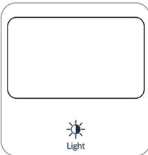
Press the Light button on the unit or remote to turn on/off the lights on the display. You can turn the lights off in any of the fan modes (Low, Medium, High, or AUTO), giving you more control over your purifier. If you power off the unit, the unit will always restart with the lights back on.
