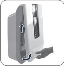
Pull the front plate toward you from its base and its magnets will release the bottom of the front cover. Then lift upward on the front plate to remove it completely, exposing the filter.
