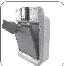
Place Filter 1 (Cold Catalyst & Activated Carbon Filter) back into the unit.
