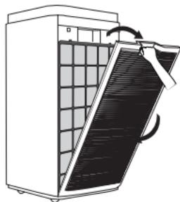
3. Take the filters out in proper order, put used filters into garbage bags to prevent contaminants from falling out.
